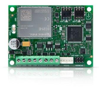
A big advantage of INT–GSM LTE device is the ability to work with the **ETHM–1 Plus** Ethernet module (RS–485 port connection). The duo allows for realization of Dual Path Reporting, in accordance with EN 50136, as well as for determining the priority of event monitoring tracks (Ethernet, cellular data and SMS). By default, cellular network is a backup communication channel for Ethernet.
