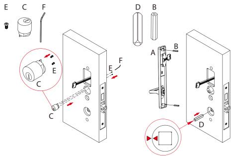
Note: Ensure the two triangles are in horizontal alignment.
