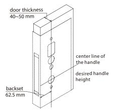
Note 1: Align the template along the vertical center line of the mortise (H) at the desired handle height, and tape it to door. Note 2: Mark the holes first, then start drilling.
